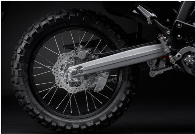
The tapered aluminum swingarm incorporates a monoblock casting that provides the correct rigidity balance and reduces un-sprung mass. Extruded aluminum is used for the chain adjustment collar.
